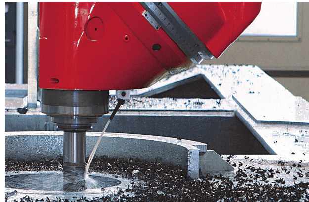
Universal milling head with infinitely variable positioning, air/oil lubrication, water-cooled, power: 38 kW, Torque: 1000 Nm, max. Speed: 8000 rpm, HSK 100-A
